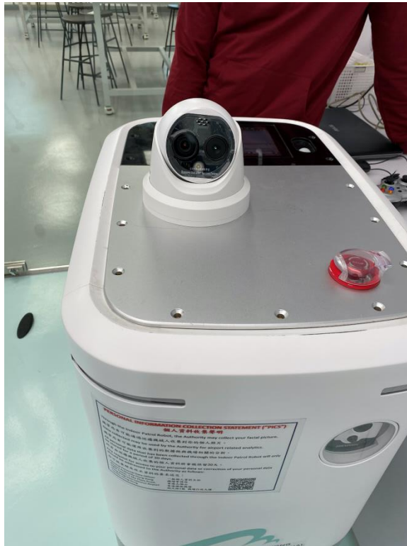
Figure 5. The patrol robot after the thermal camera is installed.
