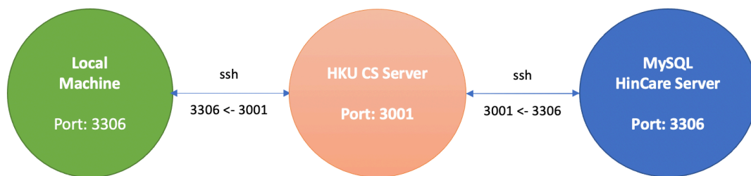
Figure 2.2.3 SSH Port-Forwarding (Tunnel)
