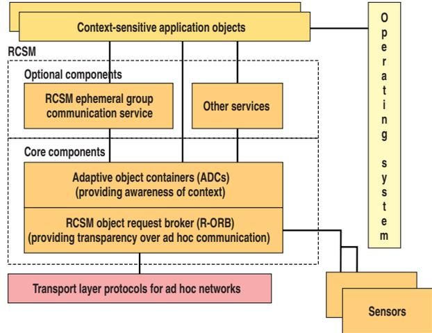
Figure 1. The device-centric architecture of RCSM (from [8]).
