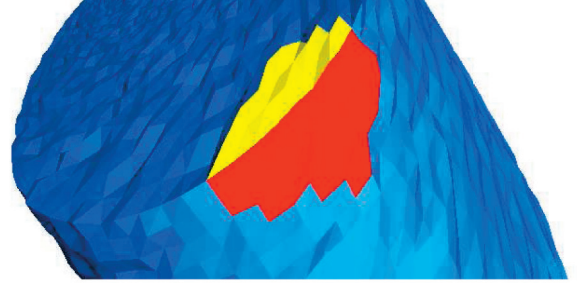
Fig. 4. Since normals in the red region have larger variations than those in the yellow region, DBSCAN is able to separate vertices in these regions into different clusters, and therefore, can achieve denoising without blurring the sharp edge between these regions.
