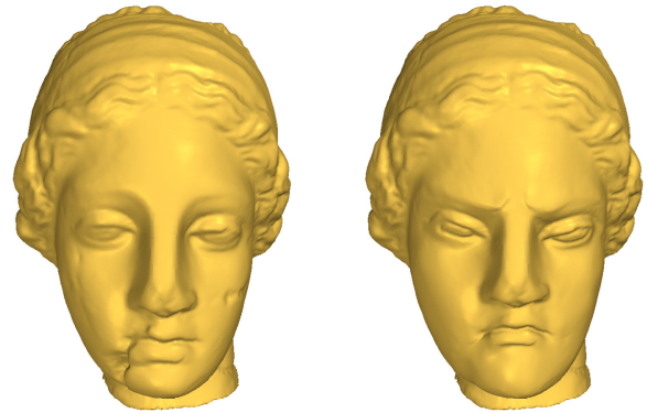
Figure 8: Left: the original Cyberware Igea model; Right: the edited model. Detail editing is applied to the eyes, eyebrows and lips to change the facial expression. Local smoothing is applied to the cheeks and the groove on the lower left part of the face.
