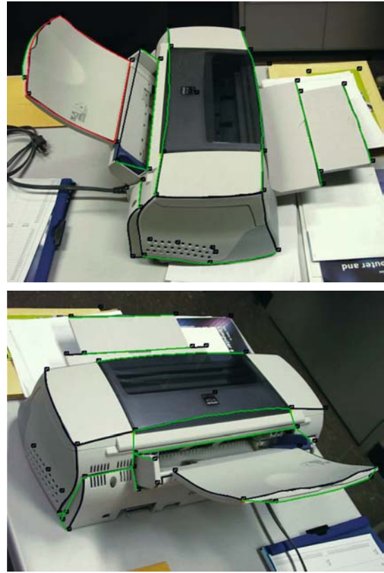
Fig. 2. During user interaction, three types of features—points, curves ( lines ) and regions—are marked. The points ( little squares ) and curves are originally drawn in black on the image planes. Their color changes to green once they are associated with correspondences. A region, shown in red, is marked by choosing a loop of curves
