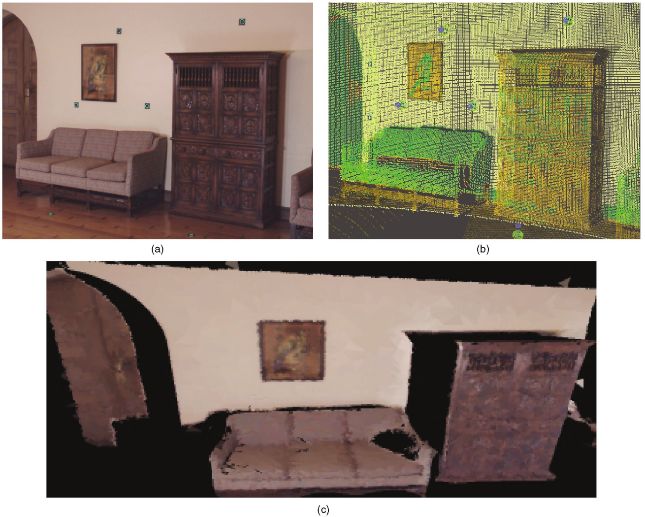
Fig. 7. (a) A real photograph with targets located. (b) The scanned point cloud viewed from the recovered camera pose. (c) Low-resolution texture-mapping using a single photograph. Note the edge alignment between the image and the geometry.
