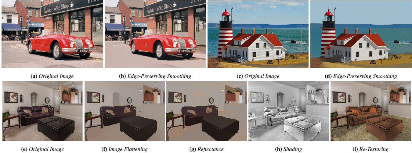
Figure 1: Our algorithm for piecewise image flattening facilitates both edge-preserving smoothing and intrinsic decomposition. Two examples of edge-preserving smoothing are shown in (a)-(d), and one example of intrinsic decomposition is shown in (e)-(h). Intrinsic decomposition enables image editing, such as re-texturing (i). Original images courtesy Flickr users 47765927@N06 (a), 132341054@N03 (c) and 37213589@N08 (e).
