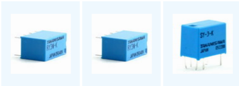
TAKAMISAWA RY12W-K Relay (2P2T, 12VDC, 960E [ ])
