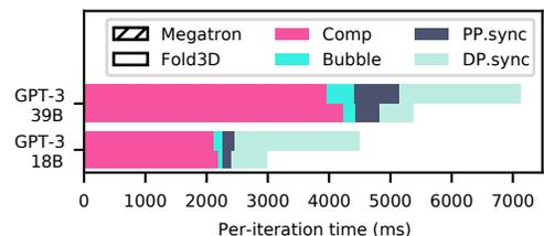
Fig. 5: Breakdown comparison between Megatron-PTD and FOLD3D. The iteration time reduced by FOLD3D matches the performance modeling in §3.3.
