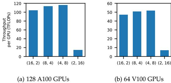
Fig. 10: Throughput per GPU under different (DP size, TP size) combinations. TP is more preferred than DP within a host.
