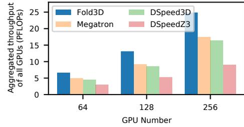
Fig. 7: Weak Scaling of FOLD3D on different amounts of GPUs. FOLD3D consistently achieves higher TFLOPs per GPU under various GPU numbers. We used GPT-3 18B, GPT-3 39B, GPT-3 81B for each amount of GPUs.
