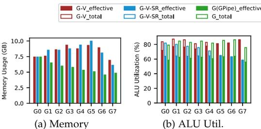
Fig. 11. Resource usage of each GPU when training (NAS-disabled) Transformer with GPipe, GPipe-vPIPE, GPipe-vPIPE-SR on 8 GPUs. Unfilled bars are wasted GPU ALU utilization for *recompute*.
