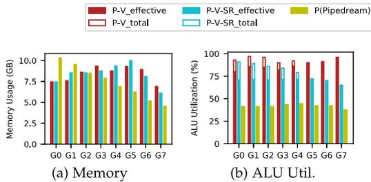
Fig. 10. Resource usage of each GPU when training (NAS-disabled) Transformer with Pipedream, Pipedream-vPIPE, Pipedream-vPIPE-SR on 8 GPUs. Unfilled bars are wasted GPU ALU utilization for *recompute*.
