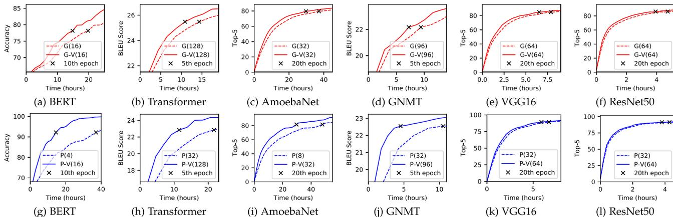
Fig. 8. Model fitting score versus time for training six models using 8 GPUs. For a-f, the models are training with GPipe (**G**) and GPipe-vPIPE (**G+V**). For g-l, the models are training with Pipedream (**P**) and Pipedream-vPIPE (**P+V**). For BERT, the score metric is next sentence prediction accuracy [10]. For Transformer and GNMT, the score metric is BLEU [58]. For AmoebaNet, VGG16, and ResNet 50, the score metric is top-5 accuracy [15], [33], [39], [44].
