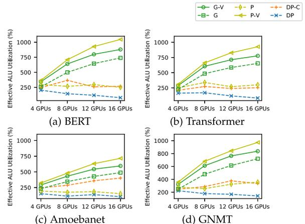
Fig. 12. Scalability. DP means pure data parallelism. DP-C means data parallelism + Capuchin [37].
