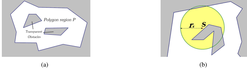
Fig. 1: Model Definition: (a) A polygon region P with transparent obstacles; (b) coverage of a sensor: the sensor S covers the yellowish area, where r_s is the sensing radius.
