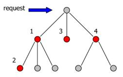
Figure 6-6: The facets to be pre-fetched in a minimal in-order pre-fetching.
