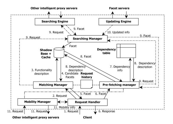
Figure 6-7: The working mechanism of a proxy server.
