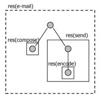
Figure 5-5: An example showing how the dynamic resource usage can be calculated by using a worst-case prediction.
