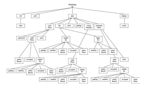
Figure 7-1: A tree showing the functionalities required by the Othello application.
