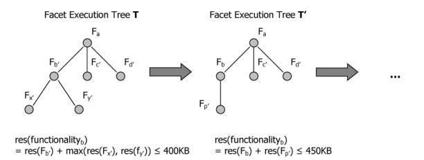
Figure 5-7: An example showing the refining of the prediction. In the execution tree T', facets  $F_a$  and  $F_b$  are known by run-time information, whereas the others are predicted with the context information at  $t_2$ .
