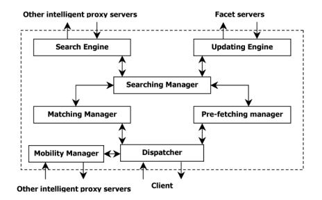
Figure 6-1: The architectural design of a proxy server.
