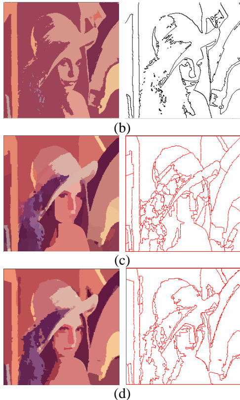
Fig.8 Segmented images and region maps of “Lenna” according to smallest L. (a) KMC. (b) SRG. (c) QBS. (d) Proposed.
