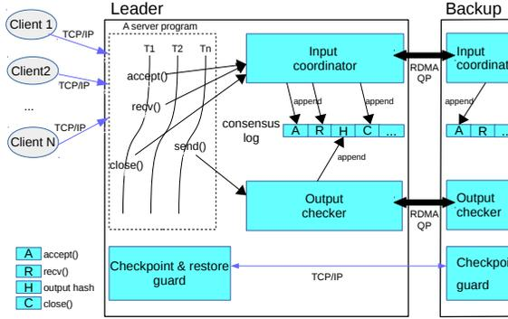
Figure 2: APUS Architecture (key components are in blue).
