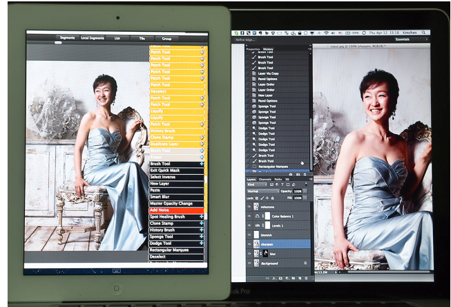
Figure 1: Data-driven adaptive history. Our system (left) provides an adaptive history with better appearance and interaction than the traditional history list as in Photoshop (right). Our prototype system is implemented as a standalone companion application (running on a tablet) for Photoshop (running on a PC), so that they display synchronized image editing state through Photoshop Connection SDK. All our visualizations (including color coding and command grouping) as well as interactions are achieved in real-time. Please refer to our video for more demonstrations.
