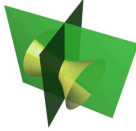
Fig. 15. The case of QSIC having two real conics intersecting in two real points.
