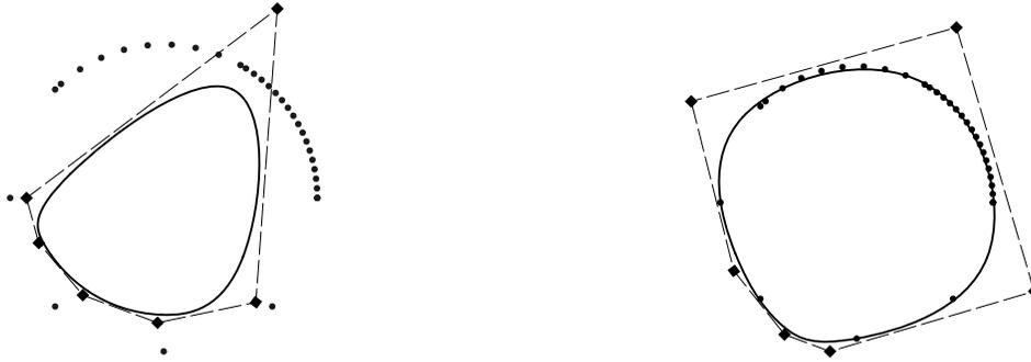
(a) Data points on a circle and an initial B-spline curve. (b) The fitting curve generated by PDM in 10 iterations.
