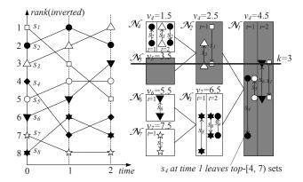
Fig. 3. Example CJI-Tree of 8 time series over 3 timestamps; 14 rank-change intervals are distributed into 7 tree nodes.
